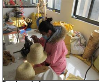
Photo of non-conformity NC - Worker in dusty working condition did not wear dust-proof mask but medical mask.JPG
